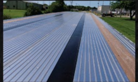
MAC Trailer proven enclosed and fully welded aluminum floor decking
