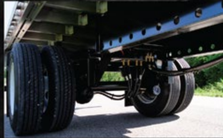
Rear axle slider suspension with pin through frame design
