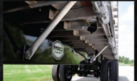
MAC Trailer proven enclosed and fully welded aluminum floor decking
